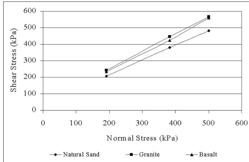
Figure 3. Strength Envelop from Direct Shear Test Results
