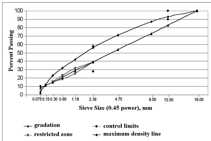
Figure 2. Gradation According to Superpave Requirements
