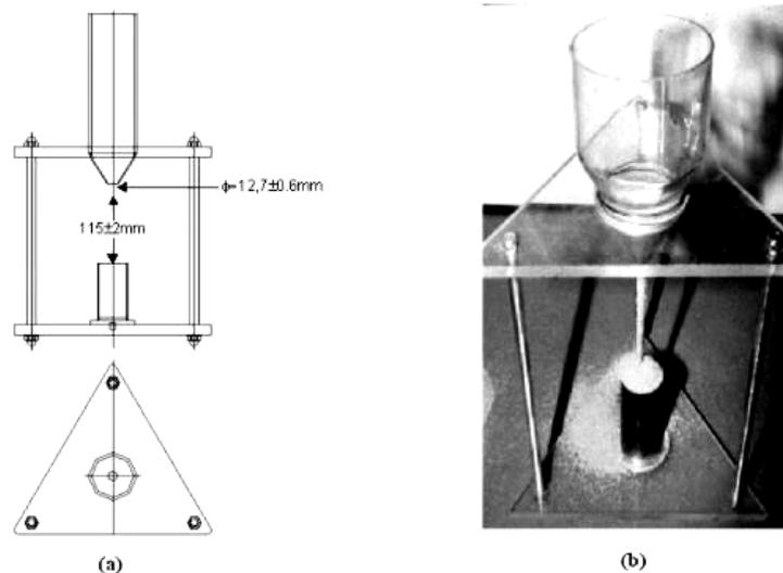
Figure 1. Fine Aggregate Angularity (FAA) Test Equipment
